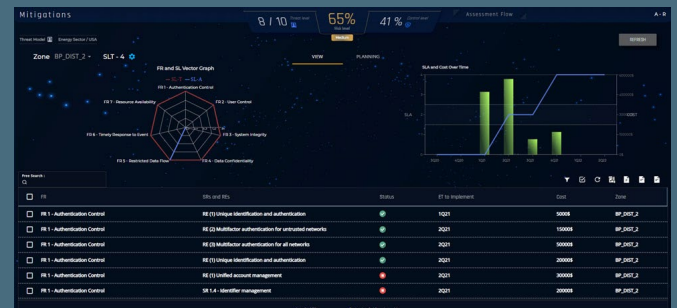
Gap-comparison between each zone's achieved (SL-A) and target (SL-T) security levels ("spider" graph, top left); controls checklist with dynamic risk scoring (bottom)
